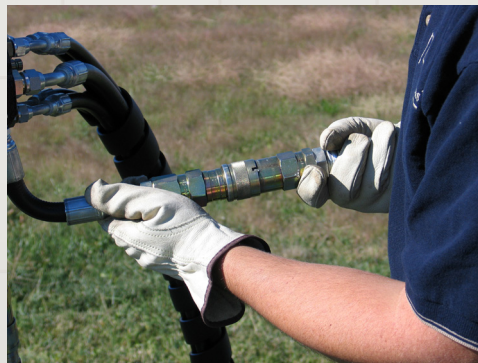
Hydraulic Quick Connects for easy & convenient set up and tear down of the 420M probe unit.
